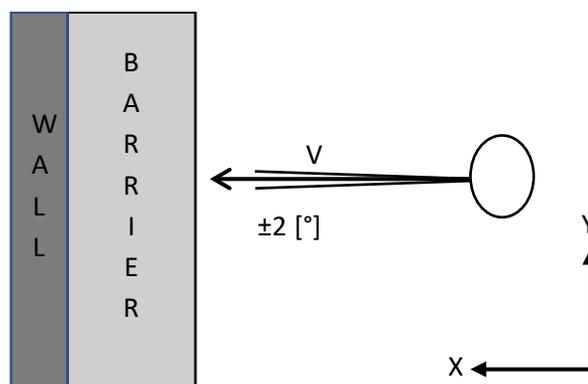
Figure 4: Top view of an impact testing
