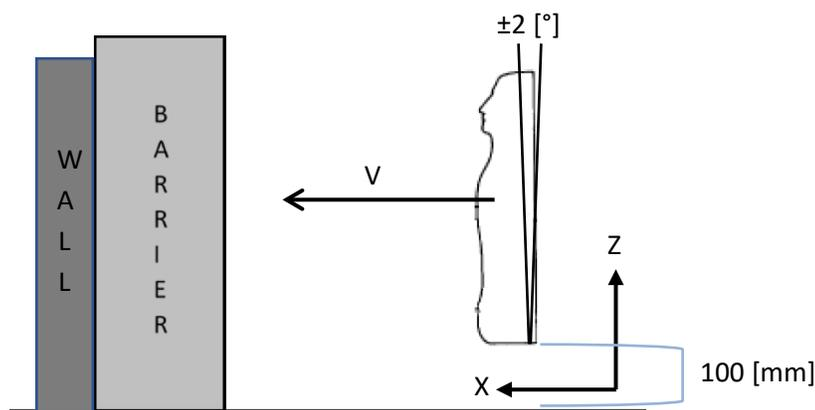
Figure 3: Side view of an impact testing
